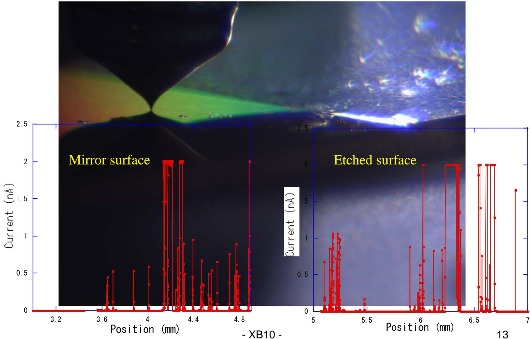
We found no surface damages after scanning on mirror surface
